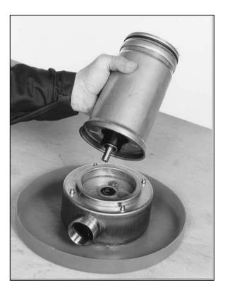
Remove the shell with stator after the oil residues have crained.
