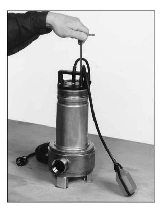
Tap the head into position with a rubber hammer, being careful not to damage it. Lubricate the thread with HT1800 or equivalent type qrease, and tighten the screws. Make sure that the washers are in place under the plastic part of each screw. (driving torque 5-6Nm).
