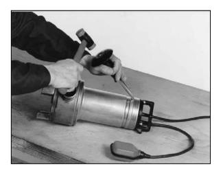
Remove the head as shown in the picture, using a plasti hammer and chisel. Be careful not to damage the head.
