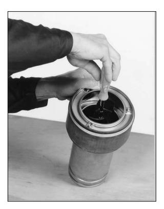
Using a socket wrench, tighten the impeller screw with its washer. (driving torque 5.5-6Nm).
