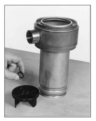
• Position the sandscreen V-ring (24) on the impeller (2); make sure that the squared side rests against the impeller.
