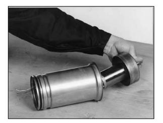
Slide out the rotor shaft and lower support. Separate the shaft from the support and remove the bearing ring (20) and the seal ring (21).
