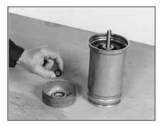
Insert the seal ring (21) over the bearing's lower support (6). During assembly make sure that the open side, where the spring is visible, is turned towards the inside of the bearing's lower support.
