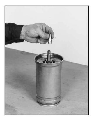
Put the mechanical seal's washer
